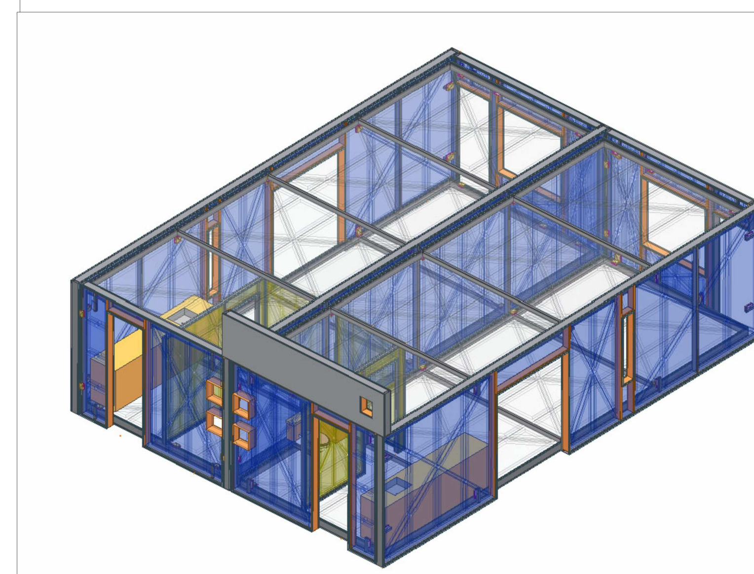
ISOMETRIC VIEWS OF THE STRUCTURAL PANELS ASSEMBLED SHOWING THE INSULATION (THAT ELIMINATES THE REDUNDANT CONCRETE) FOR WALLS, SLAB AND ROOF PANELS AND CONNECTIONS PRIOR TO CONCRETING.
